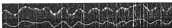
Figure 3: A single filament of false twist textured yarn's image before and after applying erosion algorithm.
